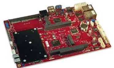
2. VersaLogic’s Viper has two Mini-PCIe sockets along with PC/104-Plus expansion.
