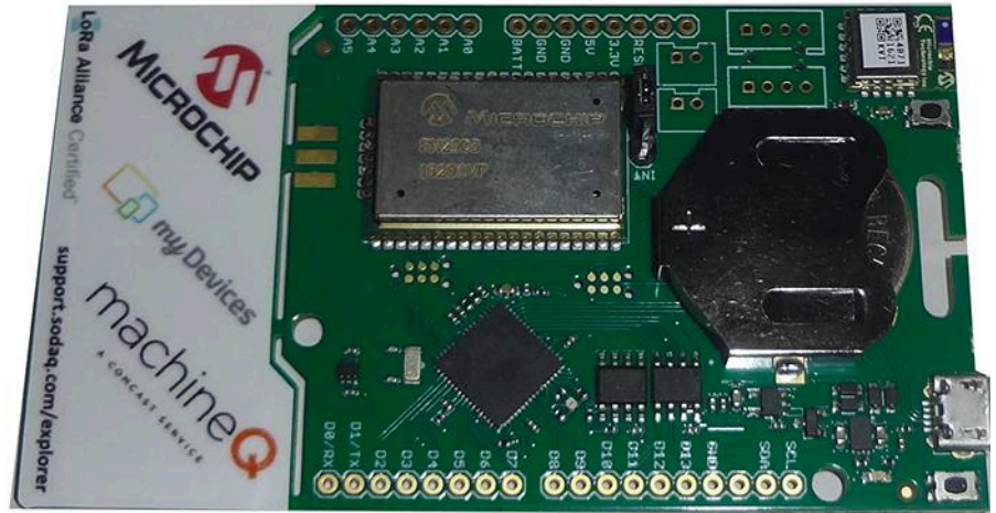
2. The Sodaq ExploRer combines Microchip's RN2903 LoRa transceiver module with its SAMD21 Arm Cortex-M0 microcontroller.
